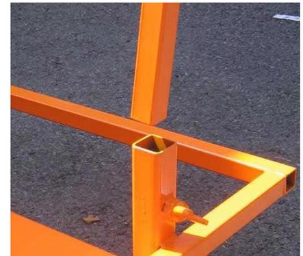
After loading the Stillage with Units hand-tighten the four wing bolts to lock the pillars
